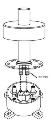
**2f.** Screw the plate onto the bottom of the faucet base with the 4 hex screws provided.
